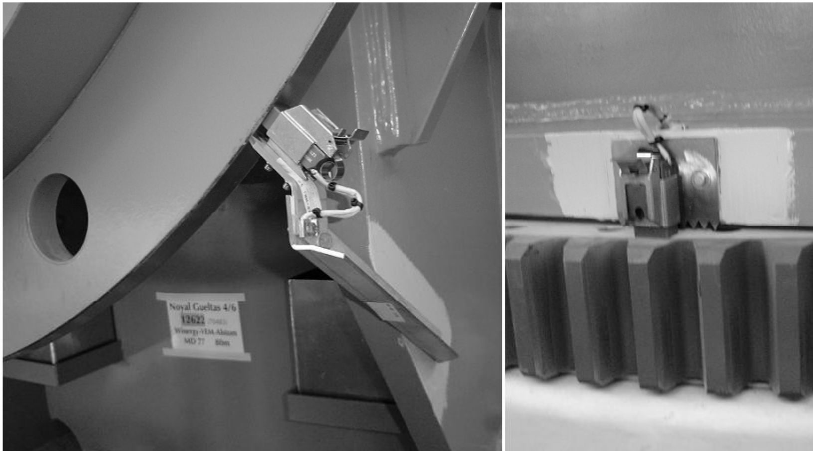
Fig. 3-47 Components of the lightning protection system for the protection of the bearings; left: sliding brush contact on the main shaft, right: on the yaw drive, combined with spark gaps (RE-power)
